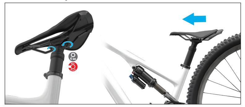
Option 2: Adjust the rear shock mount flip chip from the Low to the High position. (Approximately 6mm gain.)
